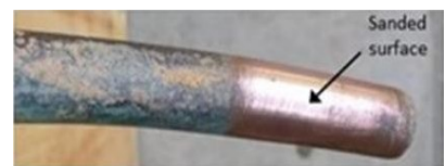
Copper looks like a new penny when scratched or sanded
