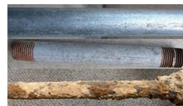
Galvanized pipes are dull gray and a strong magnet will stick to the pipe
