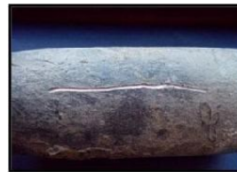
Lead pipes are dull gray and very soft and look like a new nickel when scratched or
